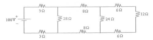
3. For the circuit shown in the figure. Calculate i) Impedance ii) Total current iii) Phase angle
