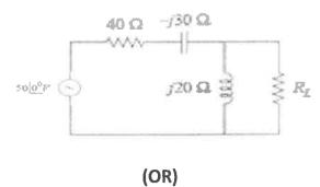
10 Find the current through load resistor R<sub>L</sub> by using Milliman's theorem for the circuit shown below?
